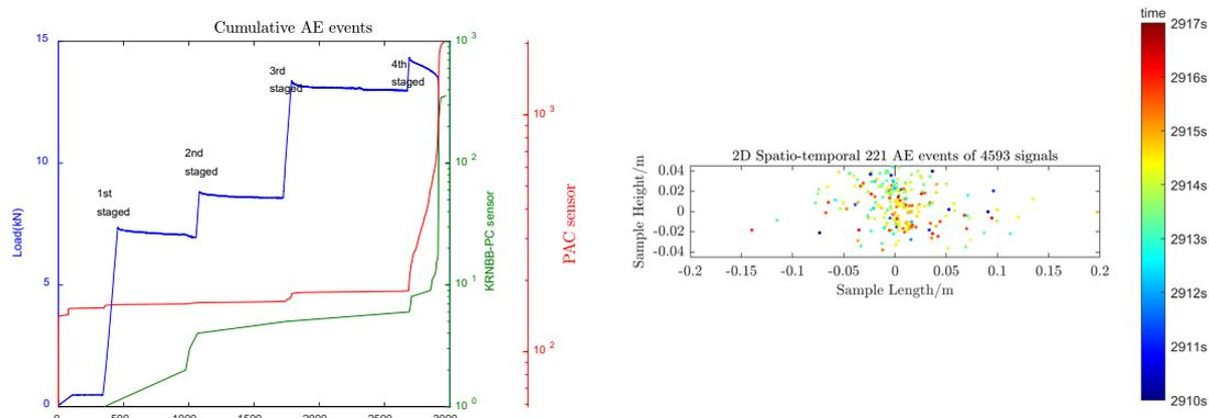
Figure 1. AE results from a SENB test. *Left*: loading data and cumulative AE events from 2 different AE sensors. *Right*: 2D AE locations from KRNBB-PC sensors during the last relaxation stage.
